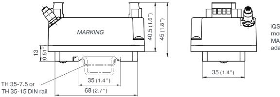
IQS910 mounted on MA130 DIN-rail adaptor
