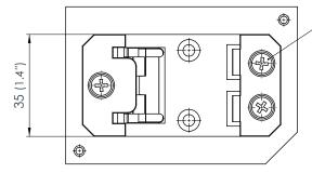
3 × self-tapping cross-head (Phillips) screws. Type: Pan-head PT<sup>®</sup> screws, H drive, 4 × 10, A2 (304) stainless steel. Mounting torque: 0.6 N•m (0.44 lb-ft).
