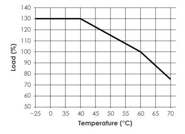
Note: Output power derating of 2.5%/°C is required for operating temperatures above 60°C (140°F).
