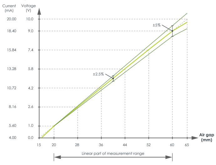
Note: This transfer characteristic curve shows the typical transfer characteristics for an LS121/ILS731 after offset compensation at 5 mm, as measured on a test bench.
