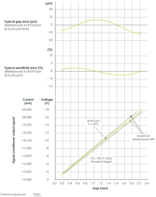
Signal conditioner: IQS900 Standard target material: VCL 140 (1.7225) Equivalent materials: A 37.11 (1.0065), AFNOR 40 CD4, AISI 4140
