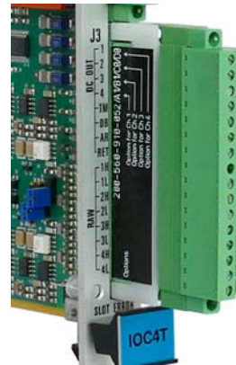
IOC4T capacitive- coupling adaptor (shown in J3 of IOC4T card)
